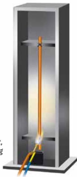
Vertical flame propagation test, self-extinguishing
