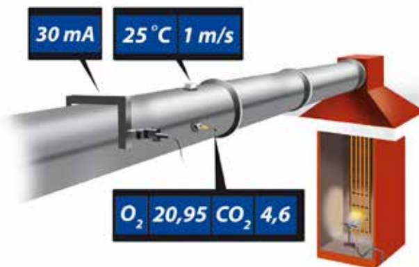
Testing the fire behaviour of electrical cables
