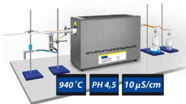
Measurement of the corrosiveness of the fire gases
